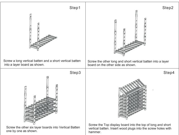
Important: When tighten the wood plugs with hammer, pls use the wood block to protect the surface of the wood plugs.
